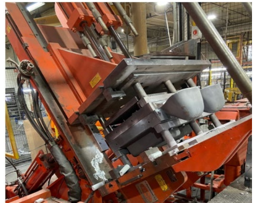
Figure 1. A tilt pour machine equipped with 10 kg (22lb) size cups. (Artwork courtesy of Paber Aluminium.)
